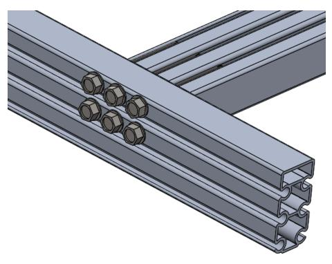
Additionally the Horizontal member can go into the lower set of channels.
